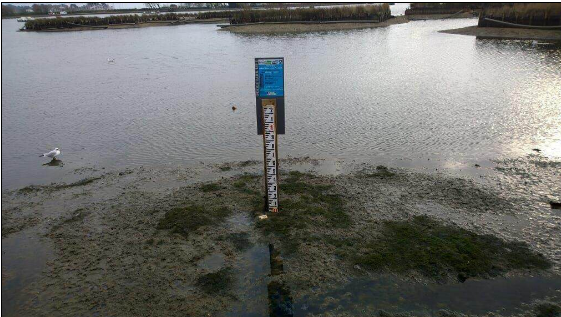
Figure 6.1 Gauge board installed in the Lagoon adjacent to The Kitchen restaurant. Photo taken at low water level during a drain down (lake full water level ~0.7 mAOD).
