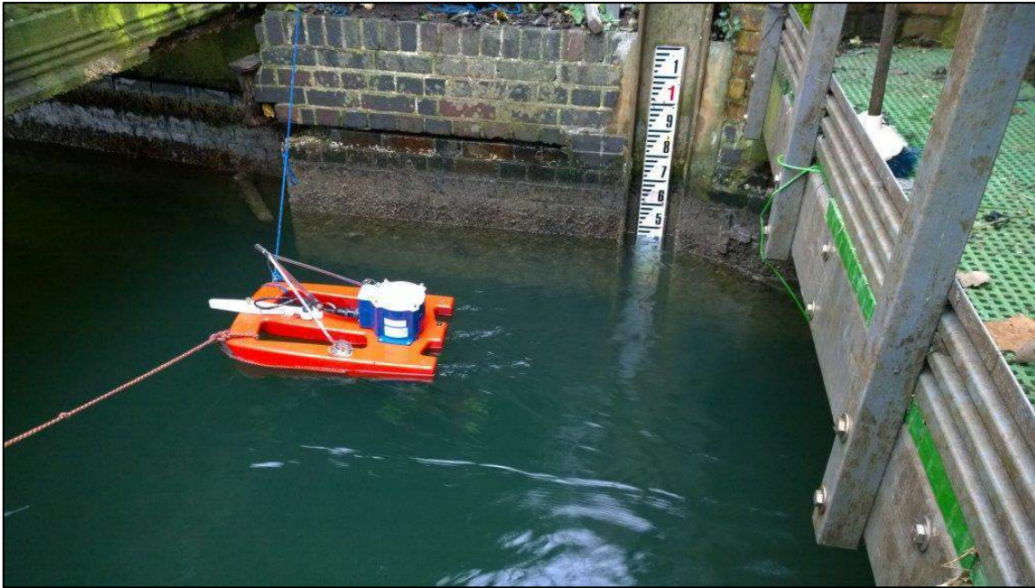
Figure 6.7 Flow gauging at the sluice gate being conducted over the full period of a lake drain down using an Acoustic Doppler Current Profiler (ADCP).
